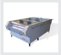
A tankless flowline system, offering water washout, drying and post exposure all in-line. A touch screen display offers easy operation, including control of the water temperature and flow speed. The proven ,plush' system that is easily adjustable, provides optimum washout results. Includes automatically lowering squeegee roll, adhesive carrier plate for foil based plates and magnetic carrier plate for metal based plates.
