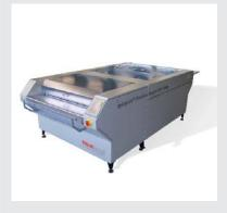
Mid-size flowline combination, offering water washout, drying and post exposure all in-line. A touch screen display offers easy operation, including control of the water temperature and flow speed. The proven, plush' system that is easily adjustable, provides optimum washout results. Includes automatically lowering squeegee roll, adhesive carrier plate for foil based plates and magnetic carrier plate for metal based plates.
